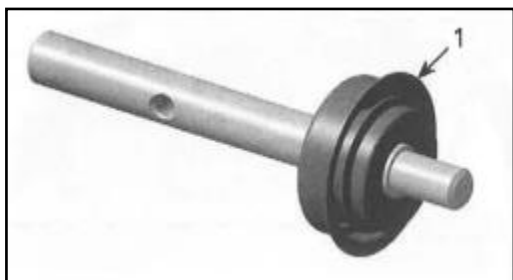
1. Surface where rotary seal is pushed by tool
