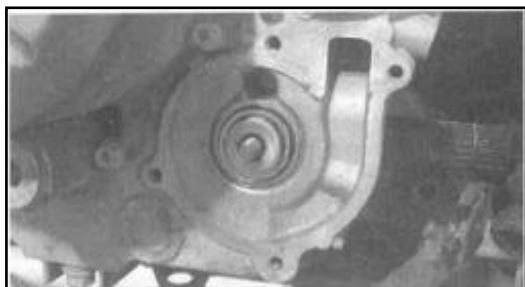
ROTARY SEAL PROPERLY SEATED ON CRANKCASE
