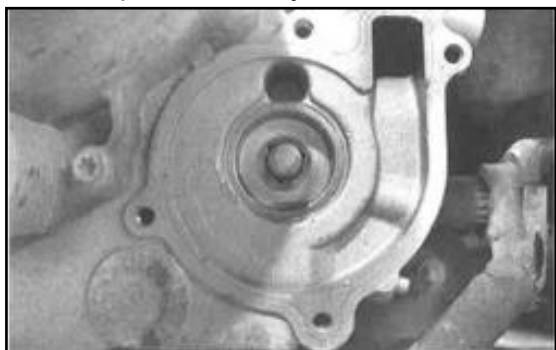
TYPICAL – INNER PARTS OF ROTARY SEAL REMOVED
