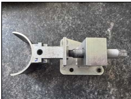
Elastic belt disassembly and assembly tooling
