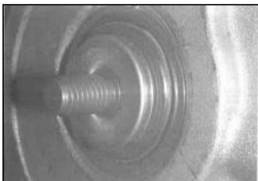
WATER PUMP SHAFT PROPERLY ADJUSTED WITH ROTARY SEAL
